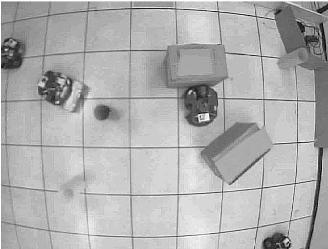
Fig. 2. Overhead snapshot of the long-term loosely coupled scenario. The robot in the center of the image is performing the cleanup task while the robot to its immediate left is performing the object-tracking task. In the upper right corner is the charging station.
